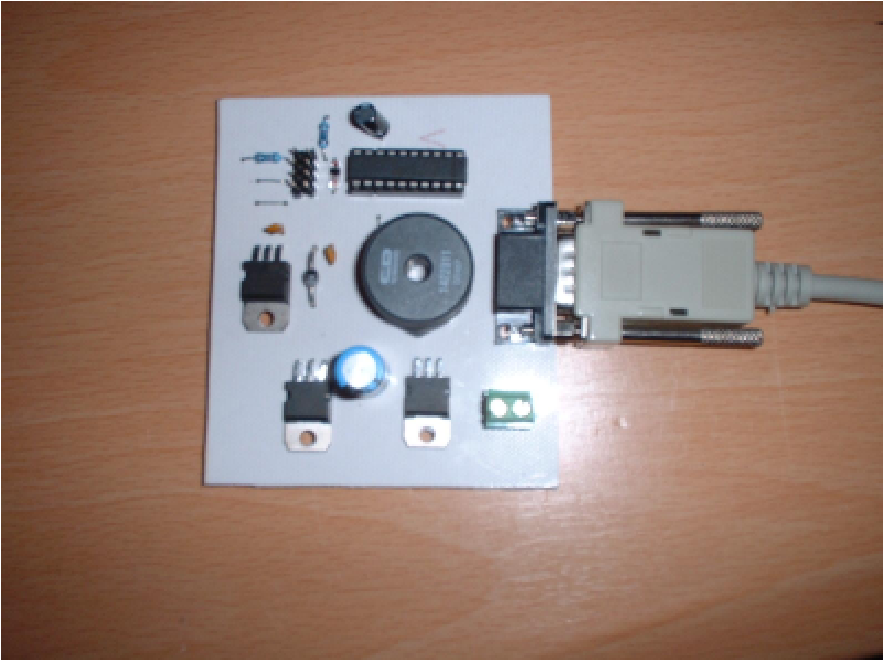
Figure 2: My first attempt at building the circuit on PCB. The inductor is rather large, but was the only one I could get with appropriate R_{DC} . My programmer circuit is connected to the PIC circuit via a 2 \times 4 IDC connector. I also used a 7805 to regulate the +5V supply to the MAX 233.
